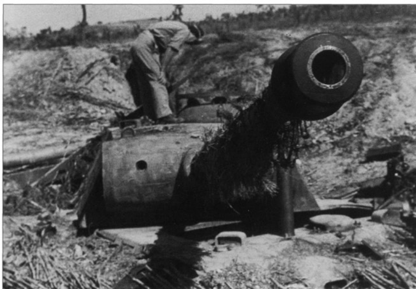
LEFT A rare photograph of one of the dug-in Panther tanks used by the Germans in the Gothic Line. Polish forces captured this example. The driver's and machine-gunner's hatches of the Ausf.A are clearly visible in the foreground. It is also possible to see the tank's original Zimmerit paste covering. (Polish Institute and Sikorski Museum)
